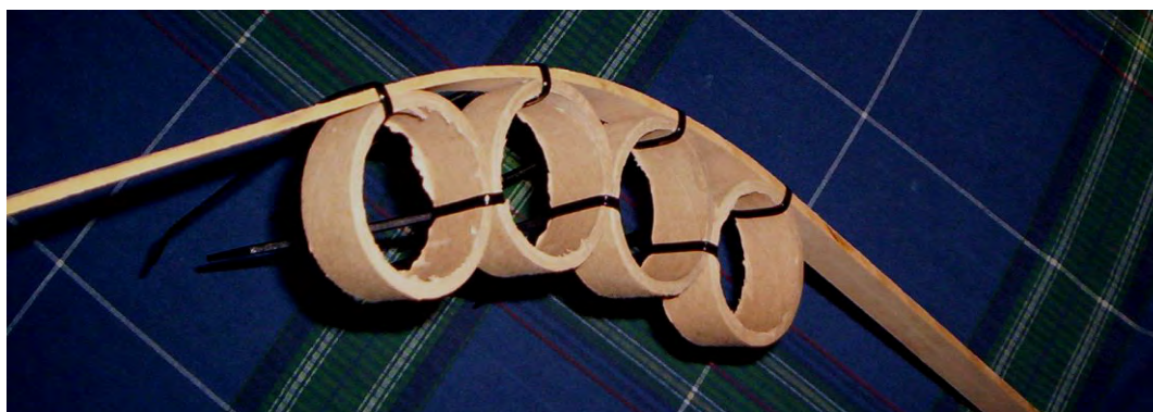
Figura 2: First Prototype laminated of MDF and tubular sections of carton.
